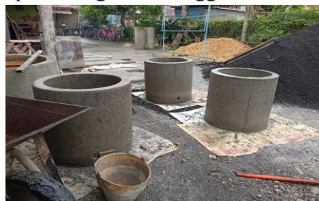
Gambar 3. Buis Beton Sumur Gali / Gorong-Gorong
