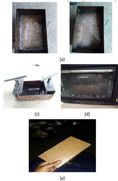
Figure 2. Fabrication stages: (a) fiber preparation, (b) fiber and polymer mixture in the mold, (c) compression molding at 250°C, (d) composite sheet after demolding
