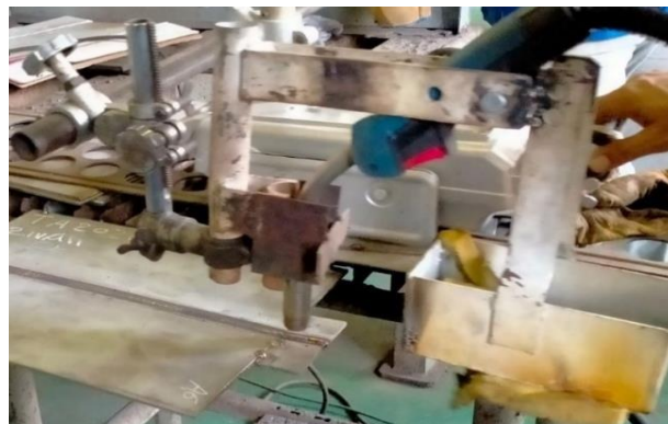
Fig. 2. Welding Scheme Using Heatsink
