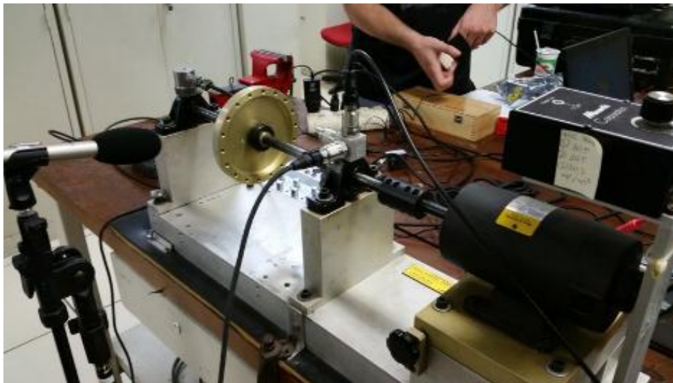
Figure 2. The acquisition device of MaFaulDa (Wang & Cao, 2023)
