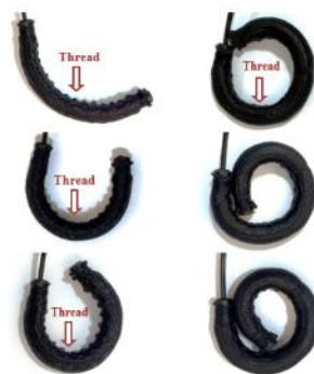
Figure 3. EBPAM pressured by different amounts of pressure
