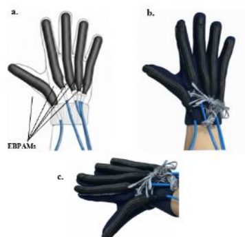
Figure 4. Proposed soft glove; (a) The design. (b) and (c) The real prototype
