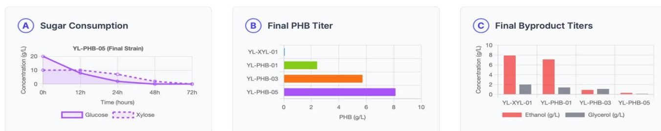
Figure 1. Performance comparison of engineered S. cerevisiae strains in shake flask cultivations on a mixed-sugar medium (20 g/L glucose, 10 g/L xylose). (A) Time-course of glucose and xylose consumption. (B) Final PHB titers after 72 hours. (C) Final ethanol and glycerol byproduct concentrations after 72 hours. Data are shown as mean \pm SD for n=3 biological replicates.
