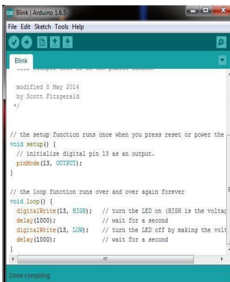
Gambar 17 : Sketch program pengujian LED
