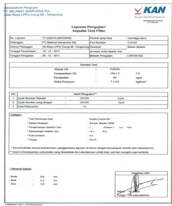
Figures 12. Report of the impulse test on the old design
