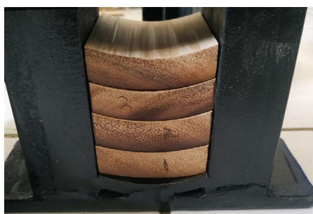
Figure 2. Laminated bamboo moulding for steam treatment
