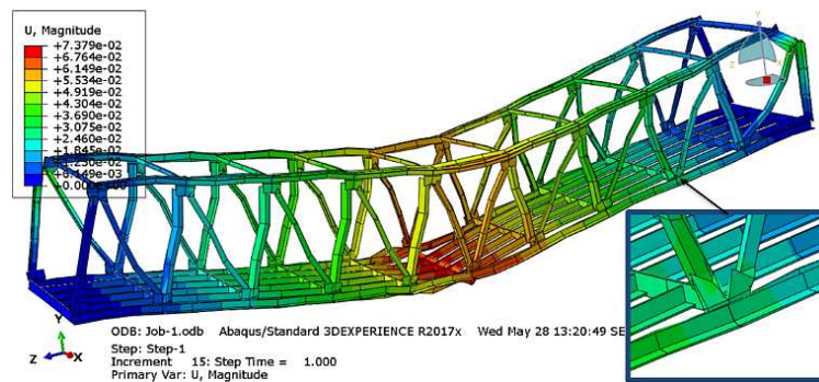
Figure 18. Bridge Modal Analysis with 5% Cutting Damage of the Gusset Plate at 1/5 of the Span
