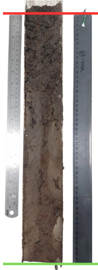
Figure 4. Sedimentary layering structure representing organic C, which is qualitatively visible by color differences. The red line indicates the upper/surface boundary (0 cm), while the green line indicates the lower boundary (50 cm).
