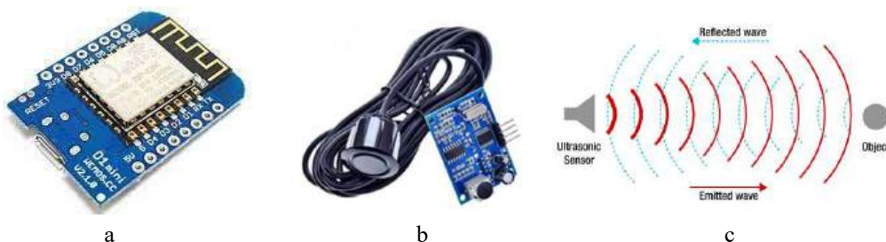
Gambar 1. a. wemos Esp-8266, b. Sensor Ultrasonic JSN-SR04T, c. Prinsip Kerja Sensor Ultrasonic
