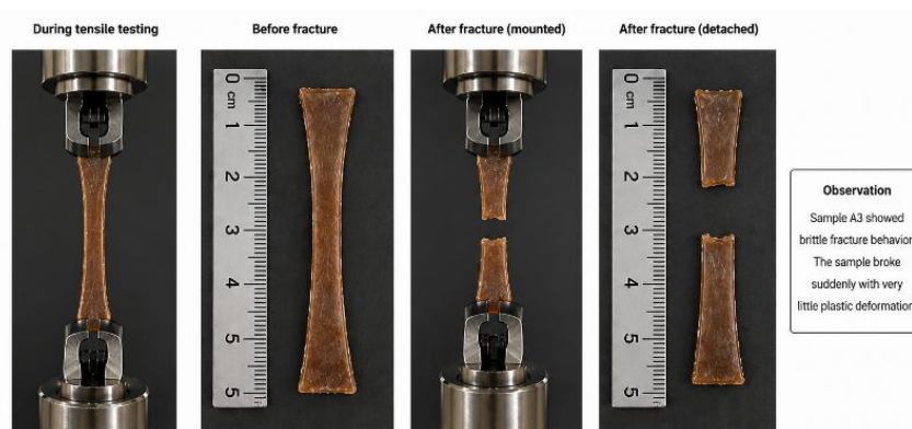
Figure 8. Tensile testing of bioplastic sample A3 (0.3 g succinic acid)
