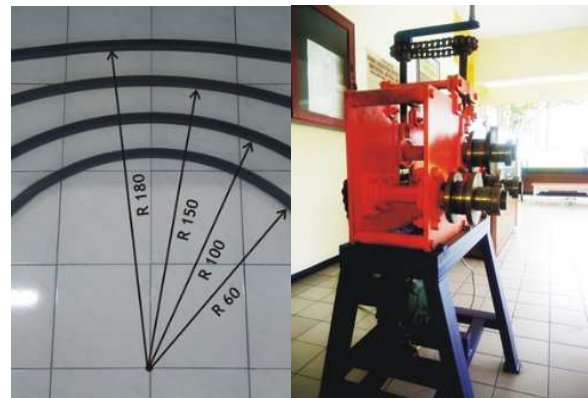
Gambar 9 Hasil curved product pada proses 3 roll bending [13]
