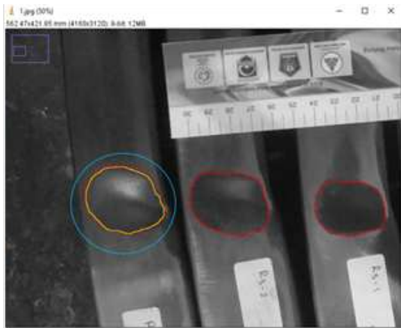
Gambar 23 Identifikasi area surface defect
