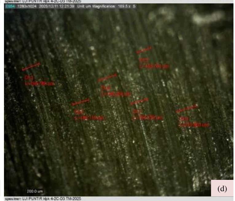
Fig. 7. Plates thickness 2 mm macro burr defect measurement. (a) 400 rpm depth cut 0.25 mm, (b) 400 rpm depth cut 0.5 mm, (c) 800 rpm depth cut 0.25 mm, (d) 800 rpm depth cut 0.5 mm.
