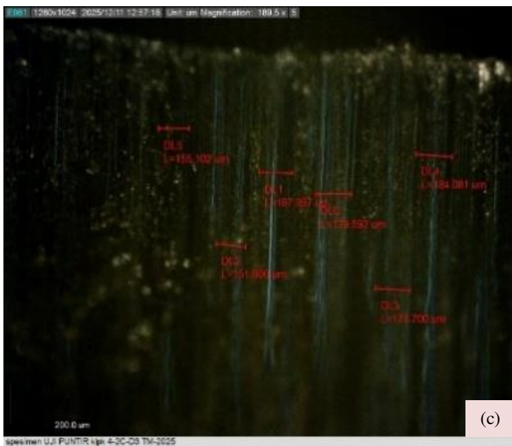
Fig. 5. Plates thickness 1 mm macro burr defect measurement. (a) 400 rpm depth cut 0.25 mm, (b) 400 rpm depth cut 0.5 mm, (c) 800 rpm depth cut 0.25 mm, (d) 800 rpm depth cut 0.5 mm.
