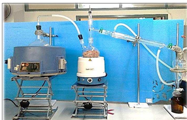
Figure 1. A typical steam distillation unit for extraction of the essential oils.
