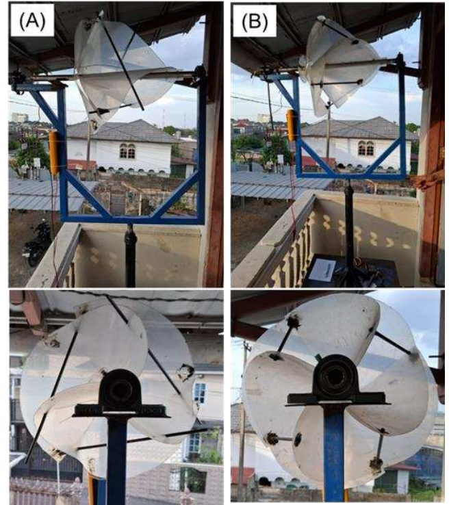
Fig 2. Photograph of the fabricated three-blade (A) and four-blade (B) ASWT
