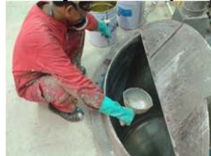
5. Flush the tank using dirty thinner.
