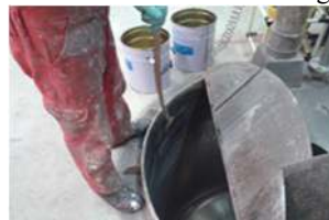
3. Scrap the tank using scrapper.
