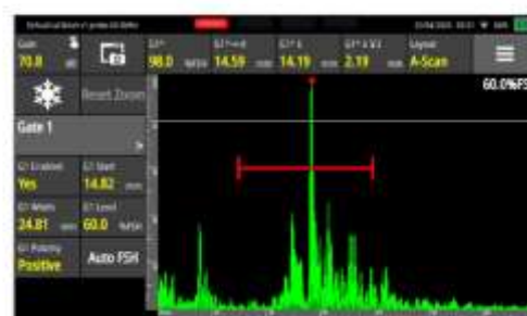
Fig. 3. Ultrasonic test results at 100 A current
