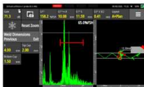
Fig. 5. Ultrasonic test results at 120 A current
