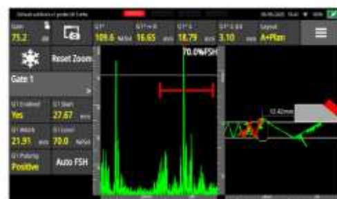
Fig. 8. Ultrasonic test results at 120 A current
