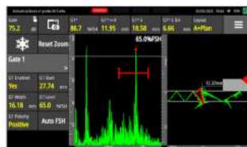
Fig. 4. Ultrasonic test results at 110 A current
