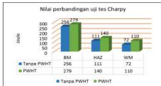
Gambar 21. Diagram Hasil Perbandingan Impact Metode Charpy
