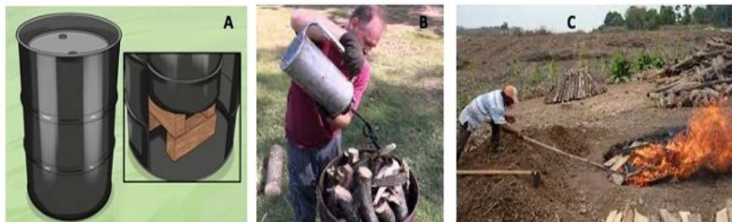
Figure 2. Charcoal production: A. Sketch of a barrel; B. Barrel method; C. Pit method
