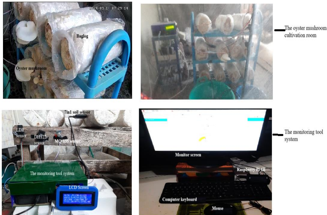
Fig. 3. Research Site And The Monitoring Tool System Of The Oyster Mushroom Cultivation Room
