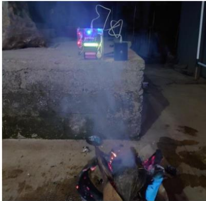
Figure 13. MQ-02 Sensor Testing
