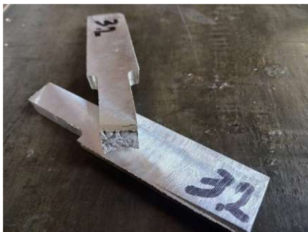
Fig. 7. The fracture of the tensile test
