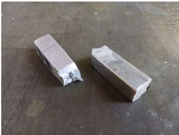
Fig. 4. The fracture of the impact test
