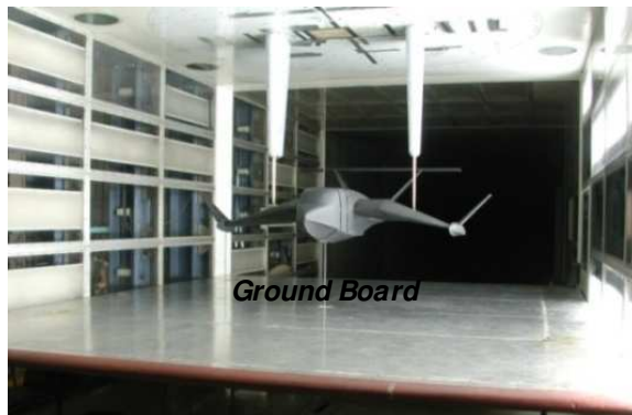
Gambar 2-2: Tes-setup model uji aerodinamik (LAGG, 2006)
