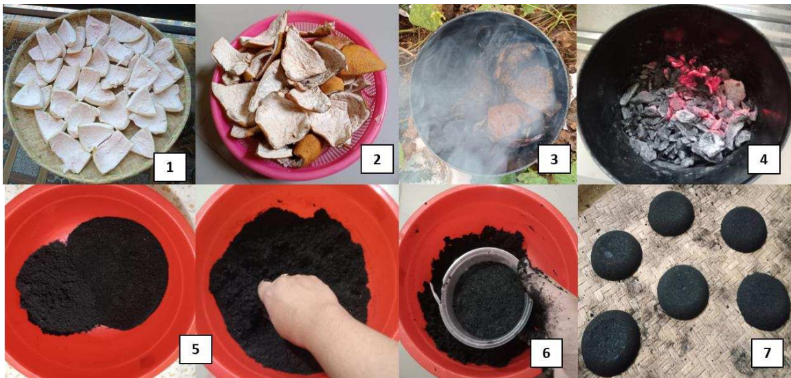
Figure 3. The instructional demonstration illustrating the sequential stages of bio-briquette production from rice husk and pomelo peel used during the technology demonstration session.
