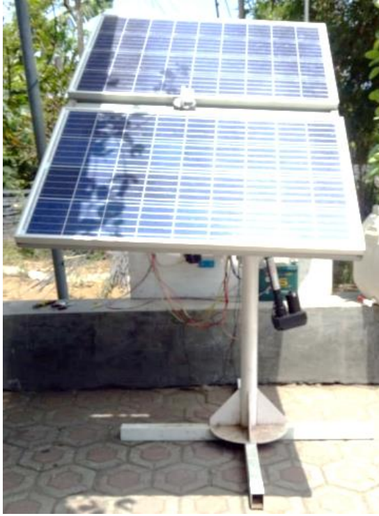
Figure 1. Design of Two Axis solar tracking PV control
