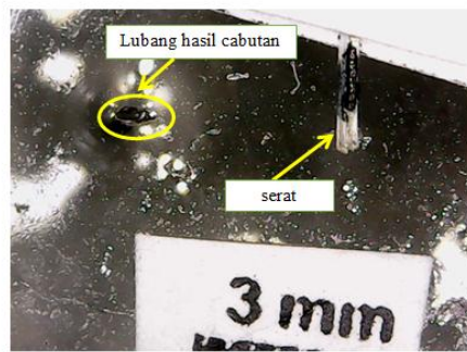
Gambar 7. Hasil uji pull out serat pandan duri tanpa perendaman
