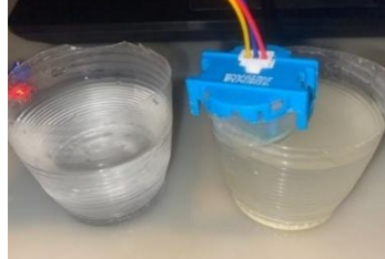
Gambar 11 Implementasi sensor Turbidity
