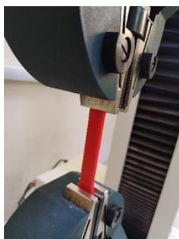
Figure 4. Tensile test of PLA+ samples.
