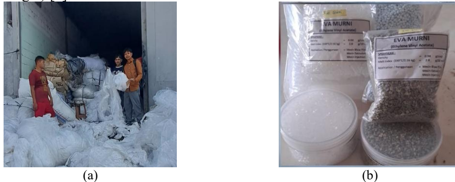
Fig. 3. Collection of EVA plastic waste and processing into plastic pellets: (a) raw EVA plastic waste, and (b) processed EVA plastic pellets.
