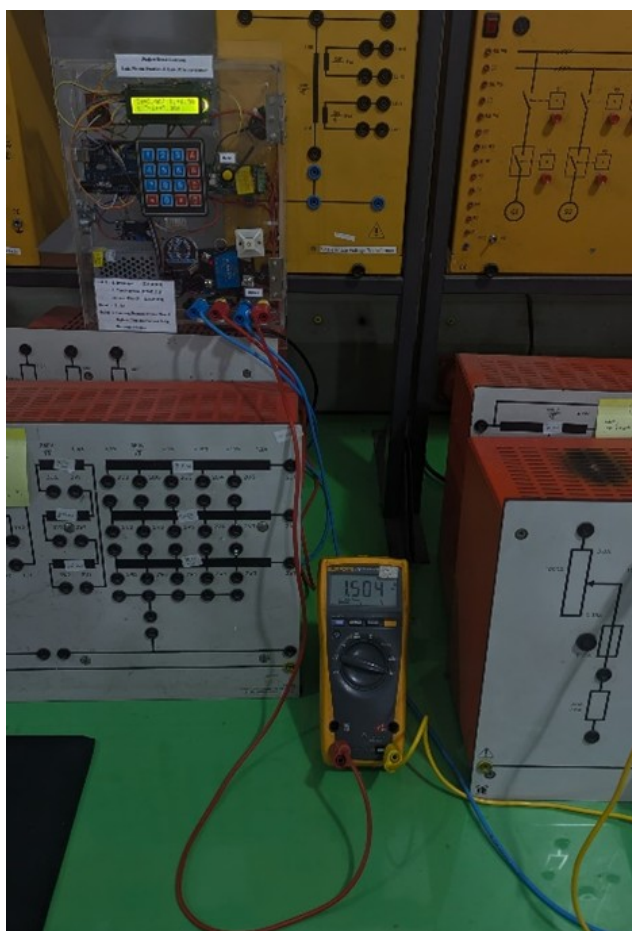
Figure 6: Inverse Time Testing with I_s = 0.5 A and t_{I>} = 0.1 s
