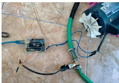
Gambar 13. Pengujian pressure transmitter sensor
