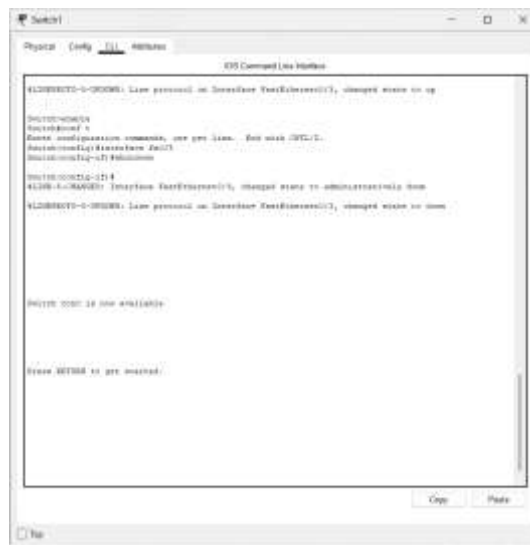
Gambar 7. Shutdown Interface Switch ke Router
