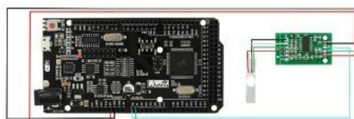
Figure 5 Schematic circuit for load cell characterization.
