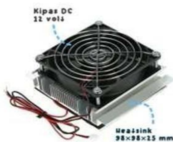
Gambar 3. Thermoelectric Generator Tampak Atas
