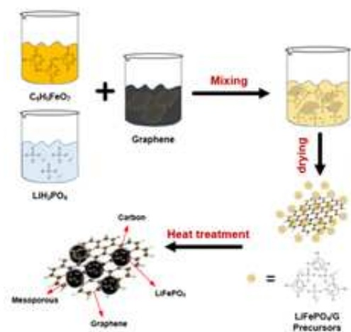
Fig. 1. The schematic of the formation of \text{LiFePO}_4/\text{VFLG} composites
