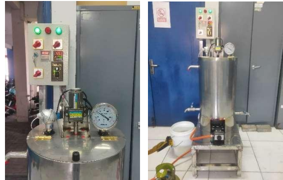
Gambar 3. Mesin Pasteurisasi Susu Sapi Otomatis berbasis Water Jacket Heating System
