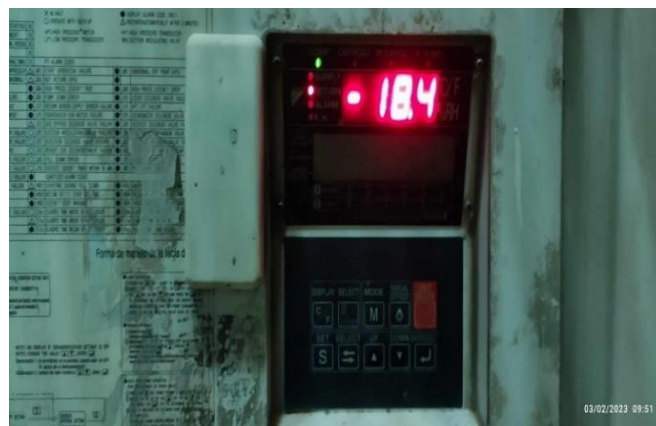
Figure 2. Temperature control box on reefer container
