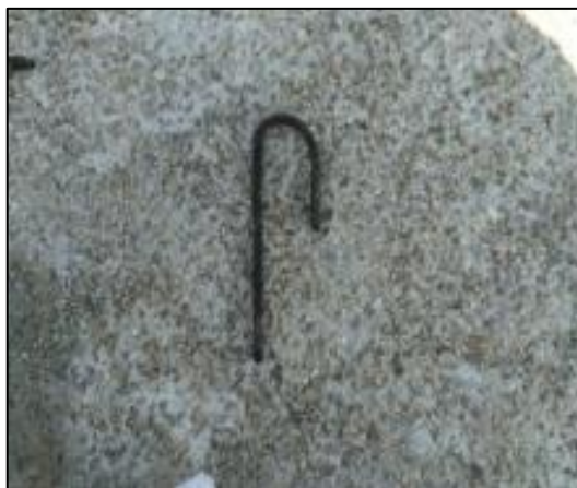
Figure 5. Plot retaining iron anchor (Permatasari et al., 2017)
