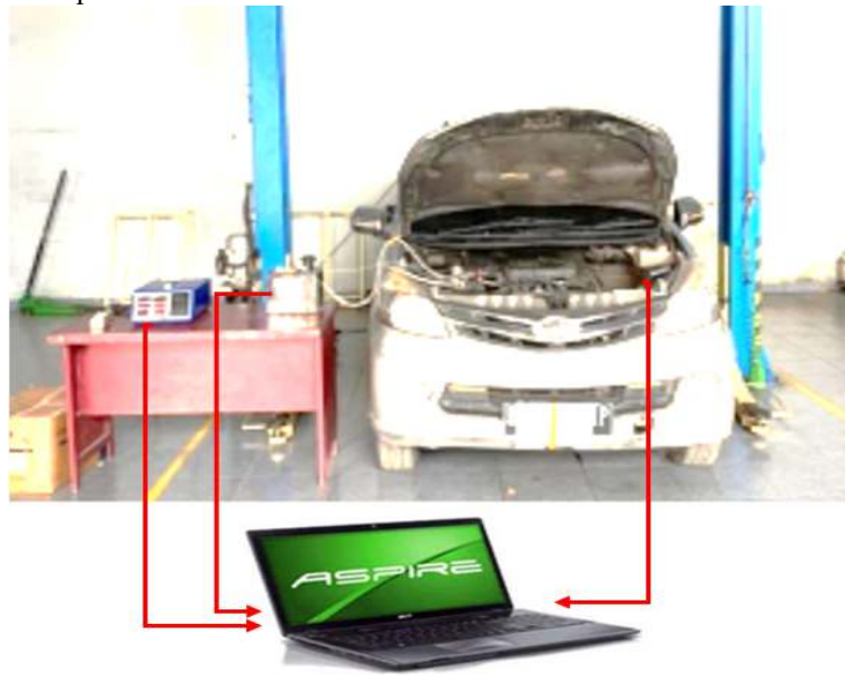
Figure 1. Experimental setup on test vehicle
