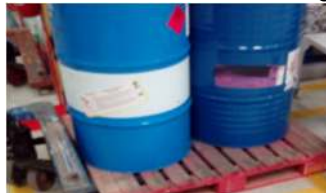
9. Accommodate the paint scale in a special drum of paint scale, lower it according to the label
