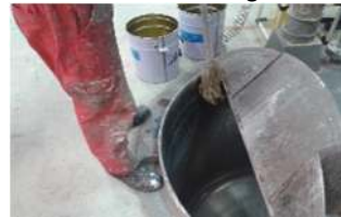
4. Re-scrap the tank using a long brush.
