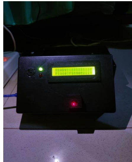
Gambar 3.2 Prototype alat monitoring bpm dan spo2
