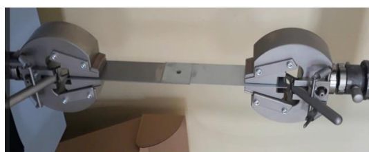
Figure 6. Tensile shear load test of the coupon on UTM
