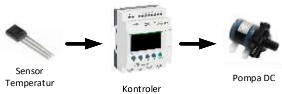
Gambar 4. Diagram blok sistem pendingin photovoltaic
