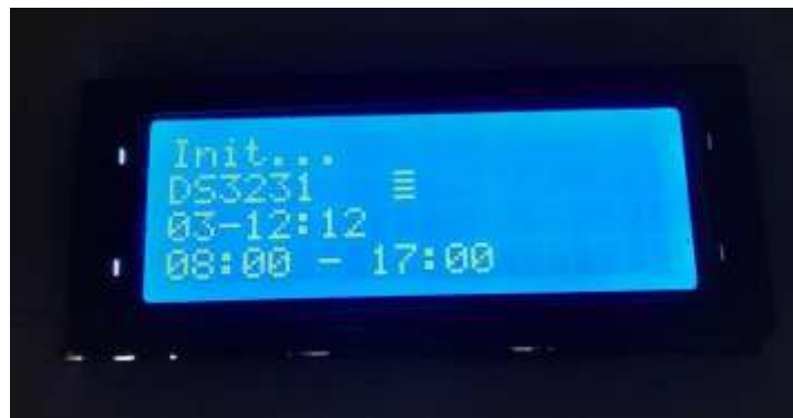
Figure 8. RTC Module Testing
