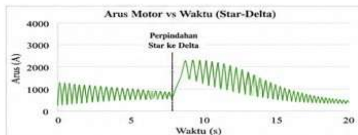
Figure 5. Starting Current Graph – Star-Delta
