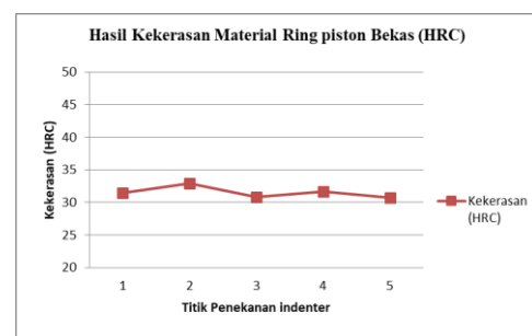
Figure 5. Hardness between used piston rings
