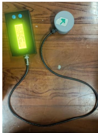
Figure 2. Prototype of IoT Sensor Test System for Building Movement Monitoring
