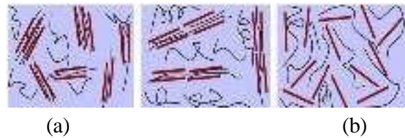
Gambar 2. a. intercalated nanocomposites ; b. flocculated nanocomposites ; c. exfoliated nanocomposites (disadur dari Suprakas, S.R. and Masami O., 2003)
